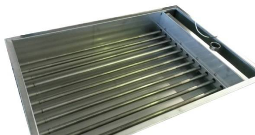
Figura 2 - heaters elements inside kettle
